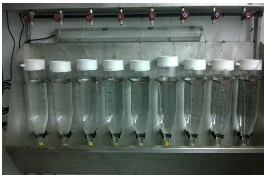
Fig. 4. Experimental system with cylindrical-conical vessels used for sea urchin larval rearing.
