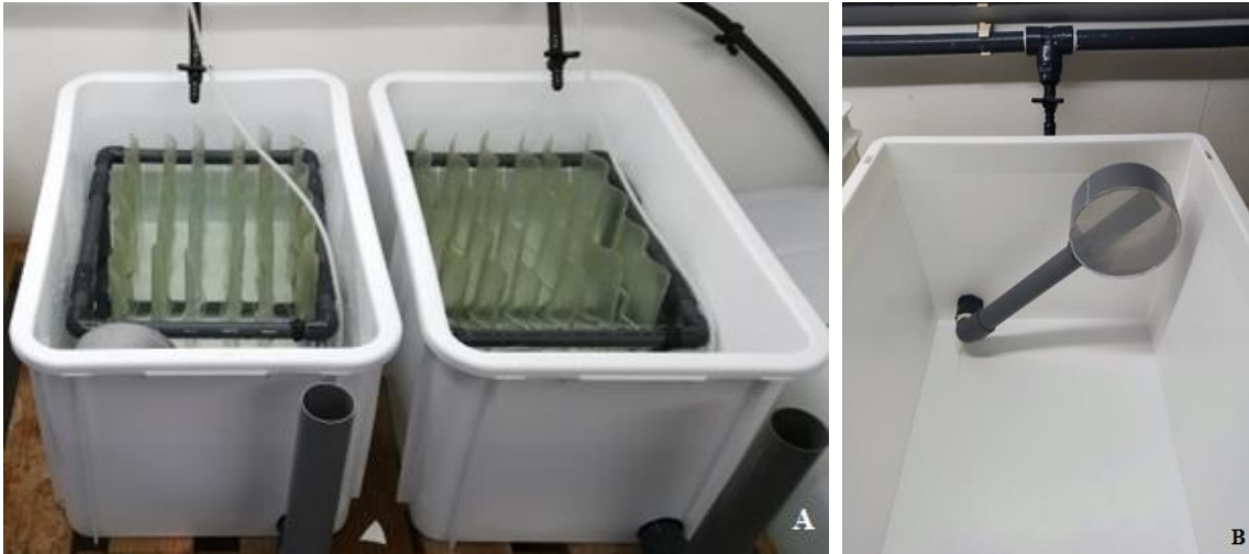
Fig. 9. Culture system used for limpet settlement and post-larval production. A. Tanks with 23 × 34 cm corrugated fiberglass plates, held vertically and at equidistant distances by the PVC supports. B. Water outlet with a 125 µm mesh sieve.
